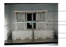
Magnetic rod holder Magnetic rod set Reagent plate (96-well deep well plate)
